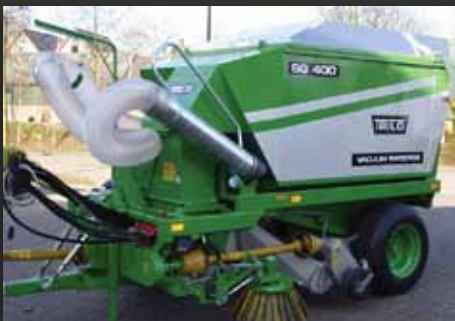
Trilo SG 400 with gulley brush and dust suppression kit.
