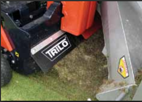
Verticutting and vacuum sweeping at the same time.
