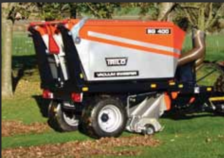
Trilo SG 400 with gulley brush and dust suppression kit.
